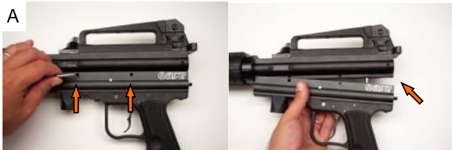
Diagram 1-2: Separating the two Body Halves.
