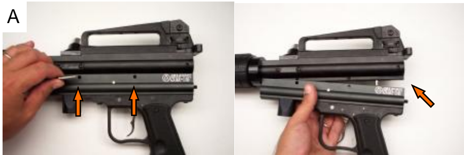
Diagram 1-2: Separating the two Body Halves.
