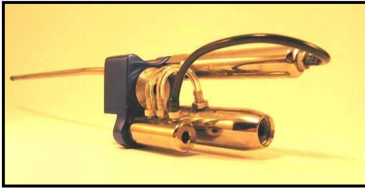
*This is what your front block and pneumatics will look like when removed from the marker. Note that the 4-way actuating rod, coupler, and spool did not come with the pneumatics. This is okay.*
