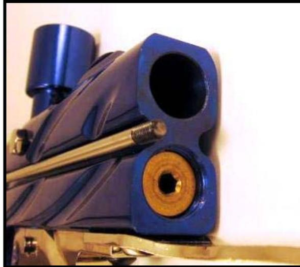
*Your marker will look like this once the Bolt, Bolt Pin, Cocking Rod, and Back Block have been removed. The brass circle in the bottom tube is the IVG.*
