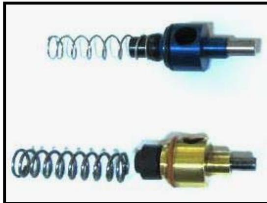
*CCM Valve Assembly – Top WGP Valve Assembly Bottom.*
