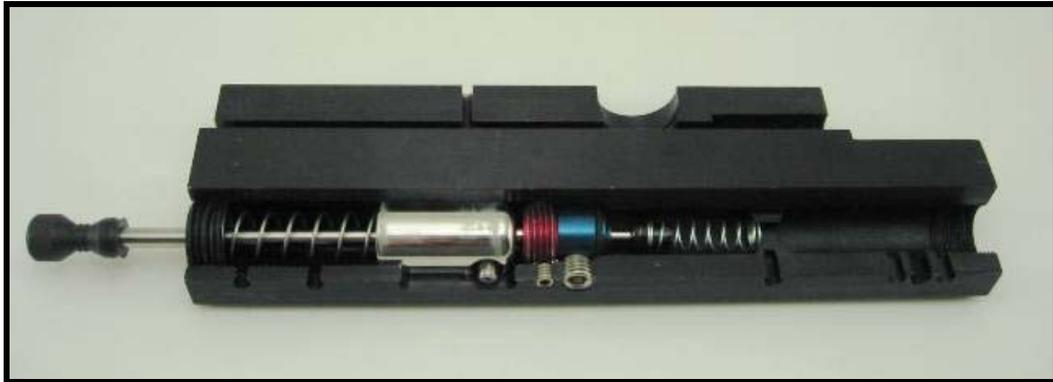
*Cutaway showing the (from left) Cocking Rod, IVG, Main Spring, Hammer (with Hammer Lug), Valve Retention Nut, Valve Body, Valve Stem, Valve Spring*
