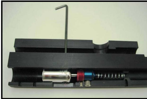
Cutaway showing the 1/8<sup>th</sup> Allen Key adjusting the Hammer Lug – shown here flush with the body of the Hammer.
