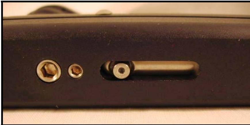
*From Left to Right: Valve Alignment Screw, Valve Retaining Nut Set Screw, Hammer (as seen through a cutout in the body)*
