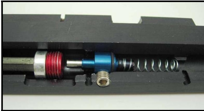
*Cutaway showing Valve Wrench removing Valve Retaining Nut.*
