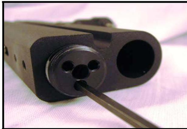
*1/8<sup>th</sup> Allen inserted in a CCM IVG.*
