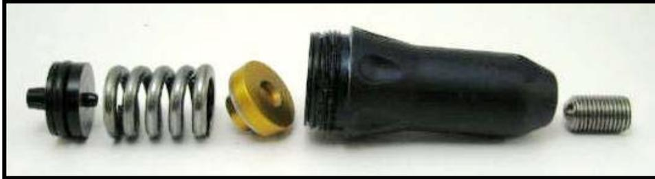
8. Clean the bottom portion and replace the Regulator piston or Regulator Piston O-Ring if necessary.
