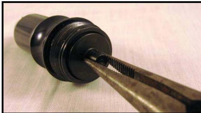
You can also take the Velocity Adjustment Screw out of the bottom and push the piston out with a longer Allen key.
