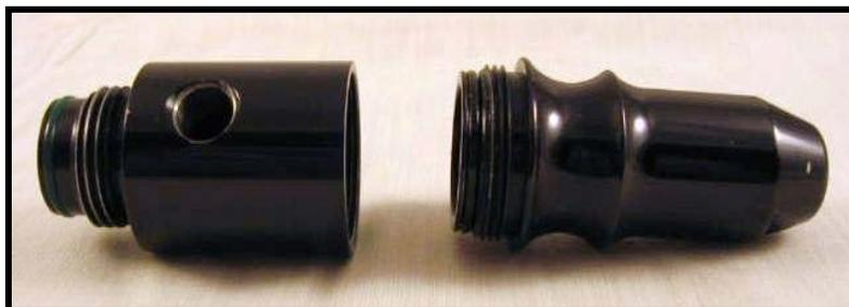
2. Use an adjustable wrench (or a 3/8<sup>th</sup> inch socket) to remove the Regulator Pin Retainer.
