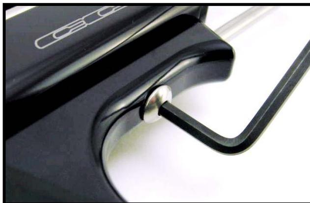
4. Remove the Auto Trigger Arm and Cam from the .45 frame. Sometimes you can simply rotate the AT arm to remove it - if it feels stuck you will most likely have to back out the undertravel screw (see below).
