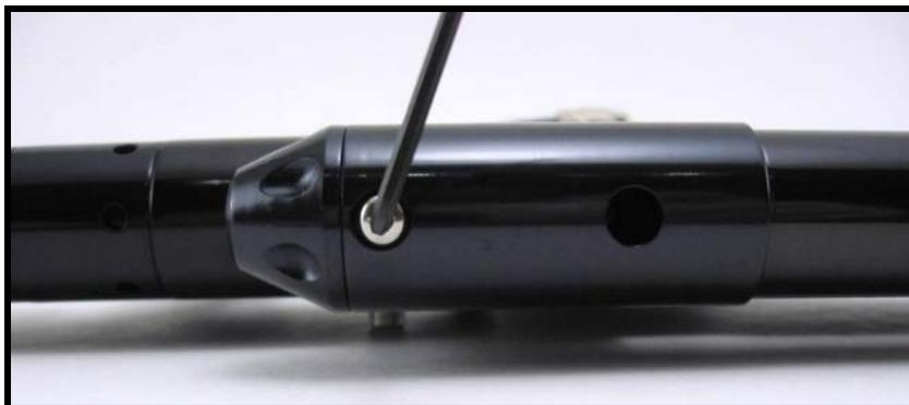
2. Remove both of the hidden screws that attach the feed to the body of the SS 25.
