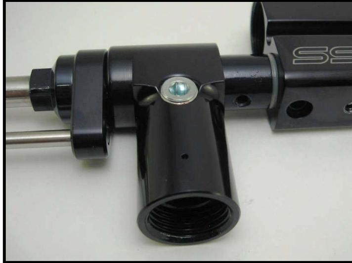
6. Note the depth of the Lug before disassembly. You want to replicate this depth upon reassembly. It will make timing the marker much easier.
