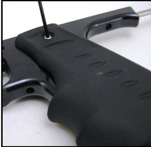
3. Remove the screws (2 1/8<sup>th</sup> Allen Screws for the SS 25 and one 1/8<sup>th</sup> and one 3/32<sup>nd</sup> for the S6P) that attach the frame to the marker chassis. The screws on the Series 6 are submerged and thus can be simply loosened a turn or two and the frame slid to the rear of the marker and removed. The Series 6 screws are of two different lengths – ensure you replace these properly when reassembling. Set the chassis aside.
