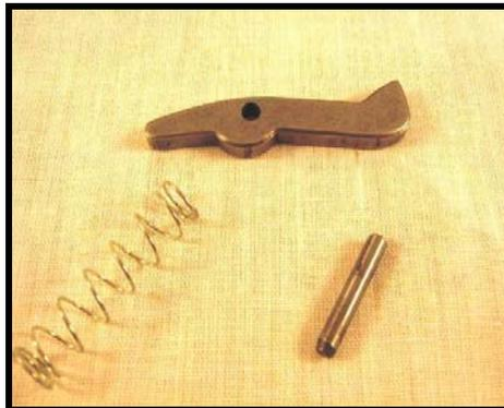
8. Inspect the Sear to see if it has wear where the lug catches. (Notice the slight wear on this sear.) Wear can cause the marker to 'skip' (not recock from time to time) or be VERY hard to time the auto trigger. Replace this if wear is evident or malfunctions are occurring. This should not need to be done often and perhaps will never need to be replaced on your marker.
