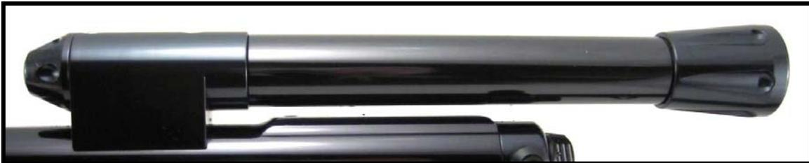
If you are lucky enough to have a Stock Class Feed Assembly, congrats because they are rare. The whole assembly only has three screws and two threaded parts. All three screws are 5/64<sup>th</sup>.
