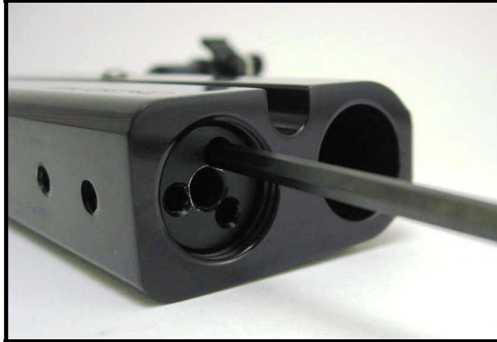
8. Insert a 1/8<sup>th</sup> Allen key into the Timing Hole (on the top of the marker) and turn the lug until it is flush with the hammer. This allows for the removal of the hammer.
