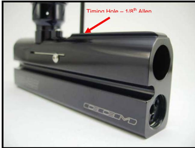
Turn the Allen key clockwise to *lower* the lug (allow the marker to fire with a longer trigger pull – or during auto trigger – later in the cycle) and to the anticlockwise to *raise* the lug (allow the marker to fire with a shorter trigger pull - or during auto trigger - earlier in the cycle).
