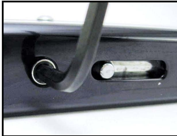
7. Remove the IVG from the marker (1/8<sup>th</sup> Allen Key) noting its depth from flush to the rear of the body. About 2 full turns or 2.5 turns are normal. The main spring will also come out at this point.
