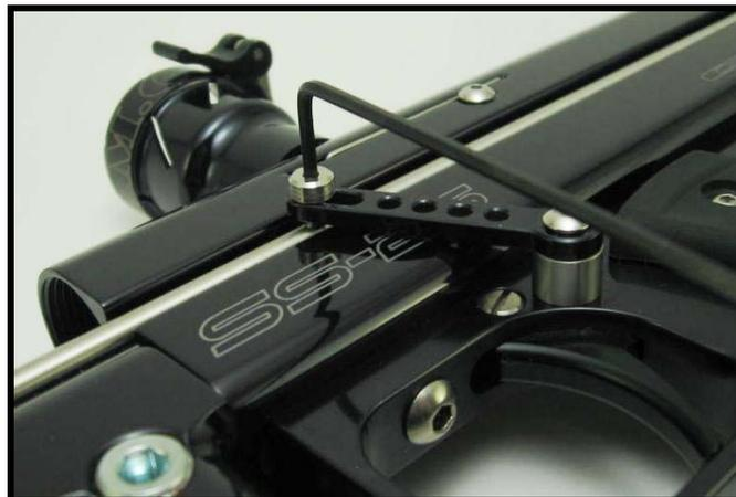
2. Remove the grip panels screws (4 - 5/64<sup>th</sup>) and the grip panels.
