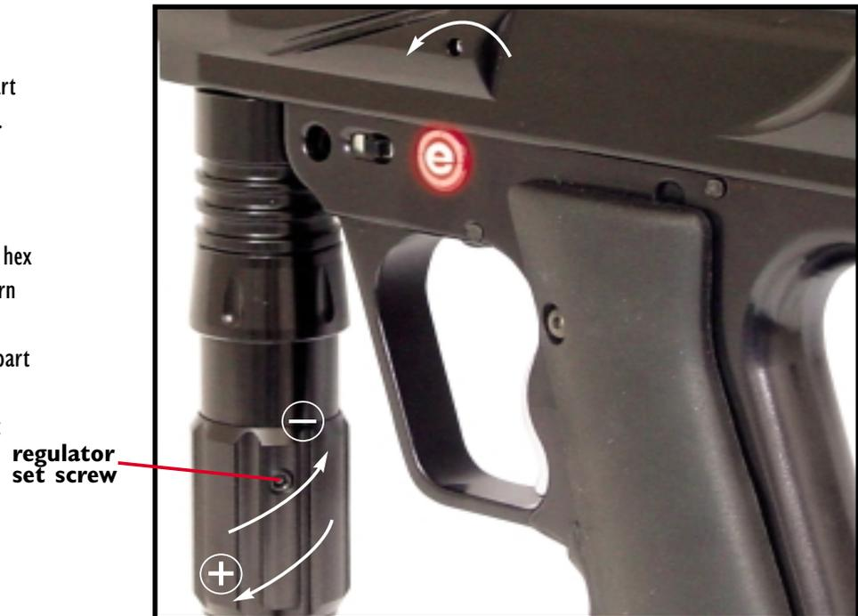
**Turn the center of the regulator to adjust pressure up or down.
