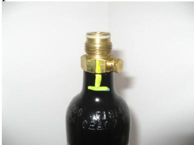
If no line is present place a non removable, non etching marking between the valve and bottle for future checks. A paint pen is a good item to use to apply the rotation indication mark.
