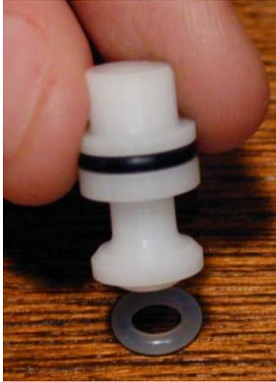
16. Drop the poppet into the O-ring setting die and drive the urethane o-ring in place by utilizing an arbor press or other significant force. Once the poppet bottoms out, do not apply any additional force.
