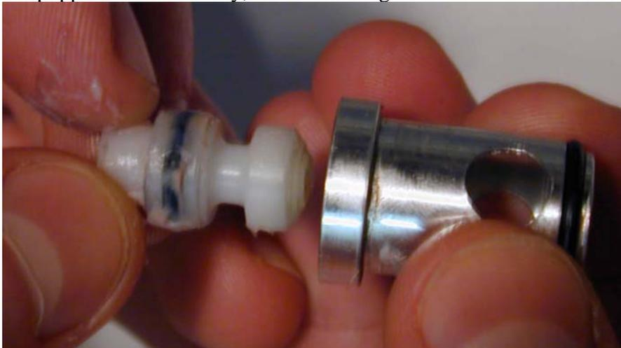
20. Put 1/2" O-ring on the front of the valve body.
