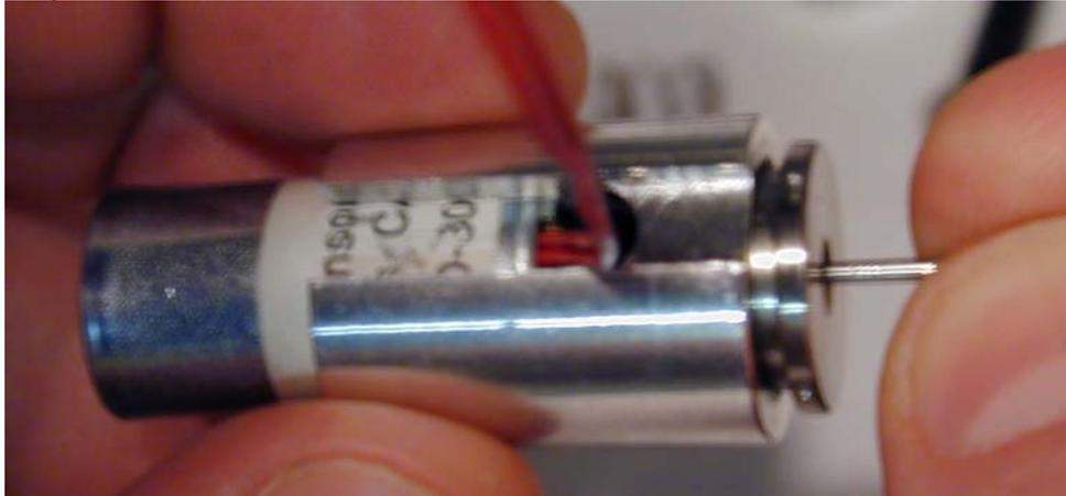
8. Loosen the orifice plate slightly by twisting the “nail” spacer back and forth.
