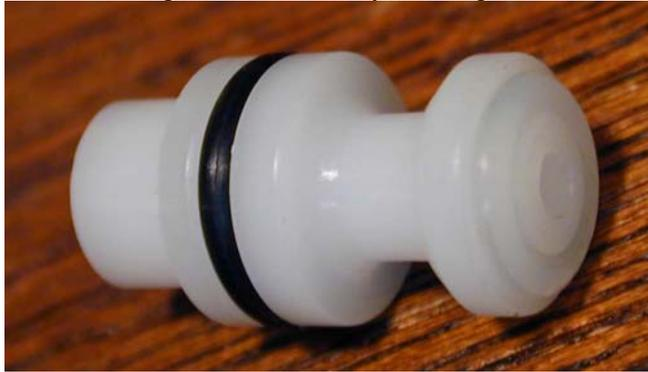
18. Lubricate the poppet with Dow 55 all over. The 3/8" buna o-ring (black) must be generously covered with grease.
