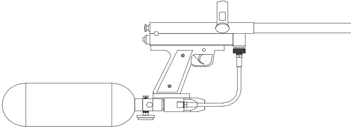
The THOR is a High Performance Second Stage Regulator that has been specifically designed to operate in conjunction with a preset primary regulator. This combination of a Preset Primary and an Adjustable Secondary provides the consistent, unvarying gas pressure and high flow demanded by the Pro Level Player.
