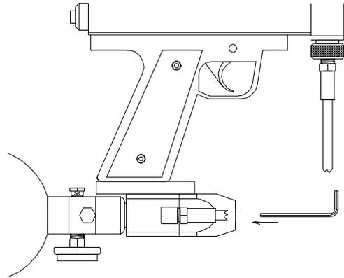
**If output pressures over 600 psi are required, insert the second shim that is supplied in the parts kit. This will move the adjustment range up to the 400 to 850 psi range.**
