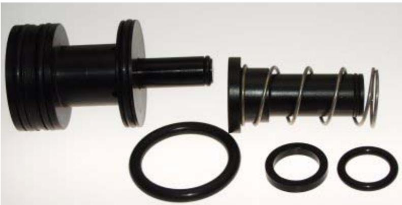
This is the most advanced ball delivery system created. Firing pressure 70-80 psi. This bolt system closes 3/4 of the firing stroke at minimum pressure to eliminate ball chopping. The last 1/4 of the bolt stroke goes full pressure to lock into closed bolt position until the ball leaves and the cycle is repeated. This is the current standard on all Assault markers. The LPR will control the first 3/4 of the stroke - approximately 7lbs closing force.
